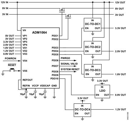
Figure 29. Applications Diagram
