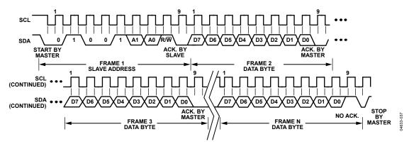
Figure 32. General SMBus Read Timing Diagram
