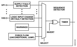
Figure 24. Sequence Detector Block Diagram
