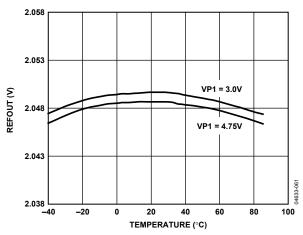
Figure 17. REFOUT vs. Temperature
