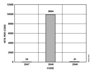
Figure 16. ADC Noise, Midcode Input, 10,000 Reads
