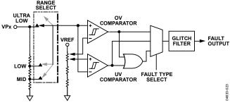
Figure 19. Supply Fault Detector Block
