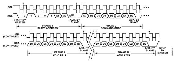
Figure 31. General SMBus Write Timing Diagram
