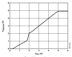
Figure 5. V<sub>VDDCAP</sub> vs. V<sub>VP1</sub>
