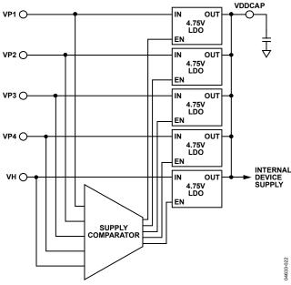
Figure 18. VDD Arbitrator Operation
