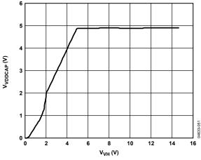
Figure 6.  $V_{VDDCAP}$  vs.  $V_{VH}$
