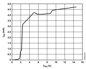
Figure 9. IvH vs. VvH (VH as Supply)
