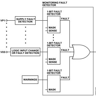
Figure 26. Monitoring Fault Detector Block Diagram
