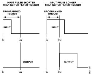
Figure 20. Input Glitch Filter Function
