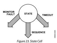
The ADM1064 offers up to 63 state definitions. The signals monitored to indicate the status of the input pins are the outputs of the SFDs.
