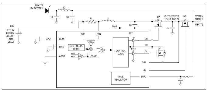
Figure 3. Boost Block Diagram
