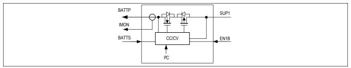
Figure 1. Charger Block Diagram
