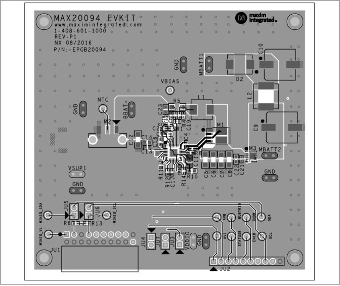
Figure 8. MAX20094 EV Kit Component Placement Guide/PCB Layout
