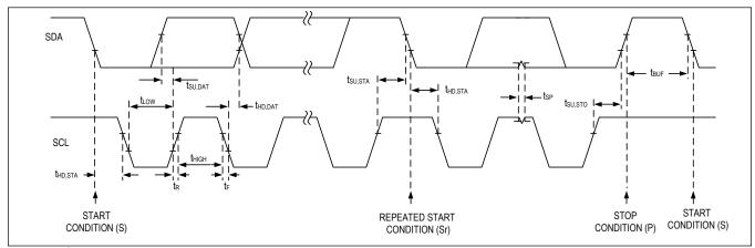
Figure 5. I<sup>2</sup>C Serial-Interface Timing Diagram
