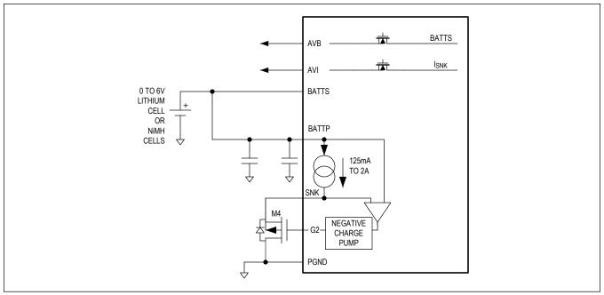
Figure 4. State-of-Health Block Diagram
