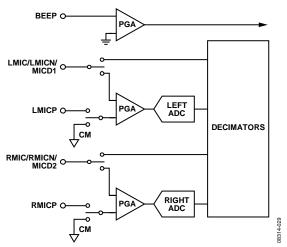
Figure 30. Record Signal Path Diagram
