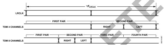
Figure 71. Example of Right Channel First, Second Pair TDM Setting
