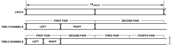
Figure 70. Example of Left Channel First, First Pair TDM Setting
