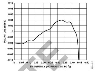
Figure 11. ADC Decimation Filter Pass-Band Ripple, 128× Oversampling, Normalized to  $f_{\rm S}$
