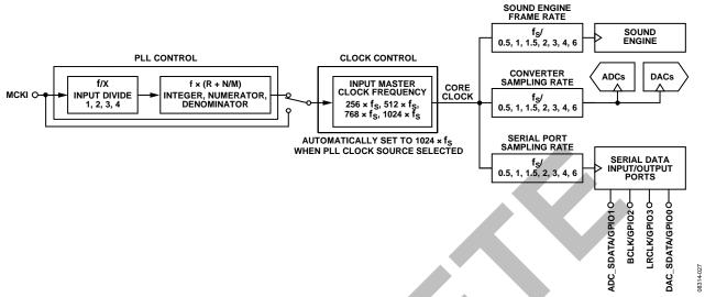
Figure 28. Clock Routing Diagram
