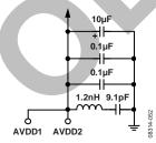
Figure 56. GSM Filter on the Analog Supply Pins
