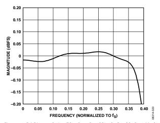
Figure 19. DAC Interpolation Filter Pass-Band Ripple, Double-Rate Mode, Normalized to  $f_{\rm S}$
