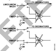
Figure 31. Stereo Digital Microphone Input Configuration
