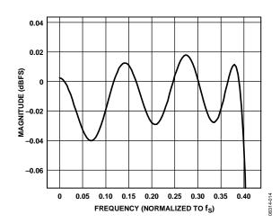
Figure 13. ADC Decimation Filter Pass-Band Ripple, Double-Rate Mode, Normalized to  $f_{\rm S}$
