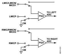
Figure 32. Single-Ended Input Configuration
