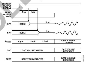
Figure 35. Speaker Driver Power-Up Sequence
