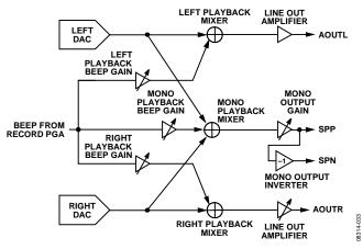
Figure 34. Playback Signal Path Diagram
