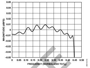
Figure 17. DAC Interpolation Filter Pass-Band Ripple, 128× Oversampling, Normalized to f<sub>s</sub>
