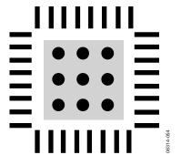
Figure 58. Exposed Pad Layout Example, Top View
