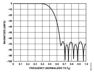
Figure 14. DAC Interpolation Filter, 64× Oversampling, Normalized to  $f_{\rm S}$
