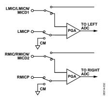
Figure 33. Differential Input Configuration
