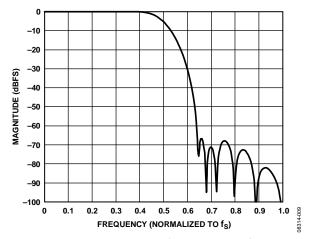
Figure 8. ADC Decimation Filter, 64× Oversampling, Normalized to  $f_{\rm S}$
