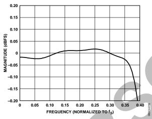
Figure 15. DAC Interpolation Filter Pass-Band Ripple, 64× Oversampling, Normalized to  $f_{\rm S}$
