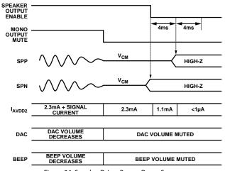
Figure 36. Speaker Driver Power-Down Sequence
