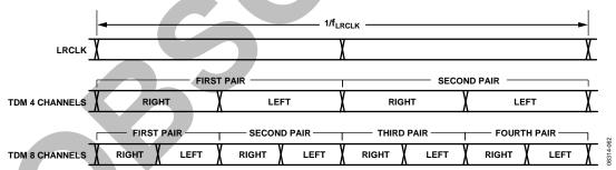
Figure 66. Right First Channel Selection in TDM
