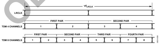
Figure 62. TDM Channel Pairs
