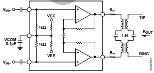
Figure 14. Typical ADSL/ADSL2+ Application Circuit
