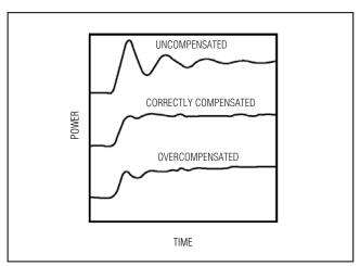
Figure 5. Laser Compensation
