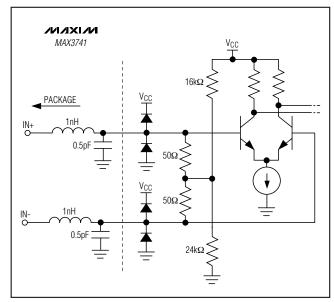
Figure 4. Simplified Input Structure
