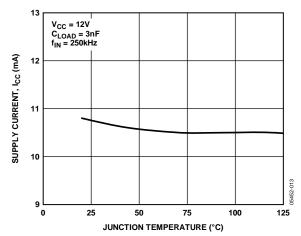
Figure 12. Supply Current vs. Temperature
