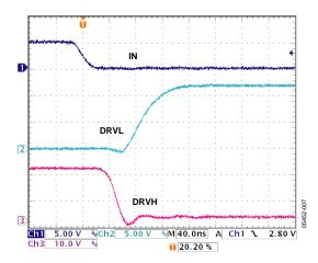
Figure 6. DRVH Fall and DRVL Rise Times  $C_{LOAD} = 6$  nF for DRVH,  $C_{LOAD} = 2$  nF for DRVH
