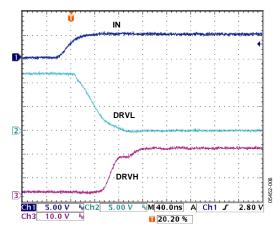
Figure 5. DRVH Rise and DRVL Fall Times  $C_{LOAD} = 6$  nF for DRVL,  $C_{LOAD} = 2$  nF for DRVH
