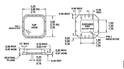
Figure 17. 8-Lead Lead Frame Chip Scale Package [LFCSP\_VD] 3 mm × 3 mm Body, Very Thin, Dual Lead (CP-8-2) Dimensions shown in millimeters
