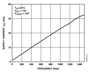
Figure 11. Supply Current vs. Frequency
