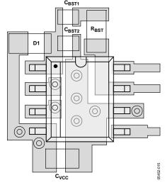
Figure 14. External Component Placement Example
