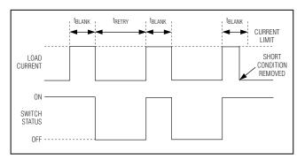
Figure 2. MAX4827/MAX4829/MAX4831 Autoretry Fault Blanking Diagram
