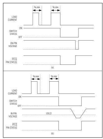
Figure 3. MAX4826/MAX4828/MAX4830 Latch-Off Fault Blanking
