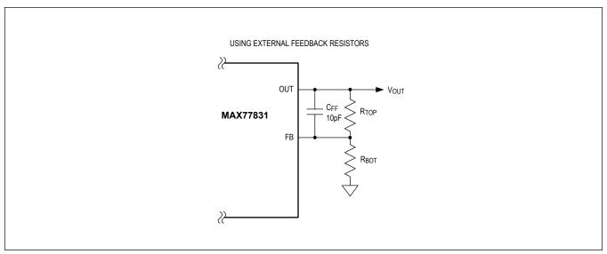
Figure 3. Connecting External Feedback Resistors to the MAX77831
