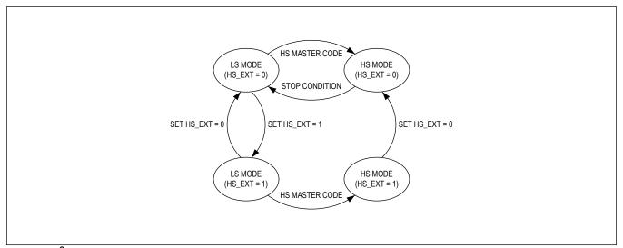
Figure 16. I<sup>2</sup>C Operating Mode State Diagram
