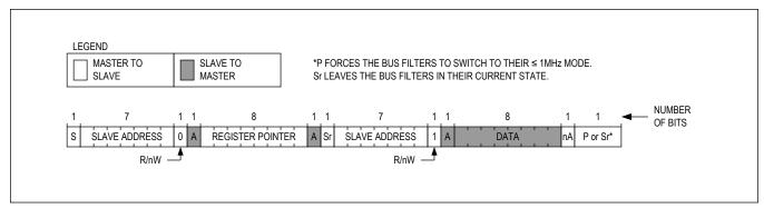
Figure 13. Reading from a Single Register
