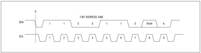
Figure 10. Slave Address Byte Example
