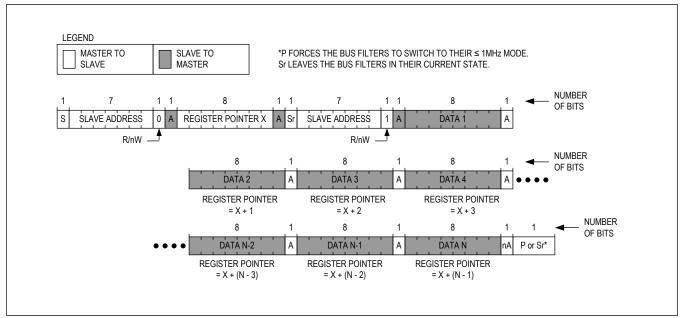
Figure 14. Reading from Sequential Registers
