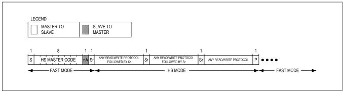
Figure 15. Engage in High-Speed Mode Protocol
