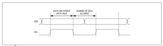
Figure 7. I<sup>2</sup>C Bit Transfer
