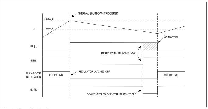
Figure 5. Thermal Shutdown Recovery
