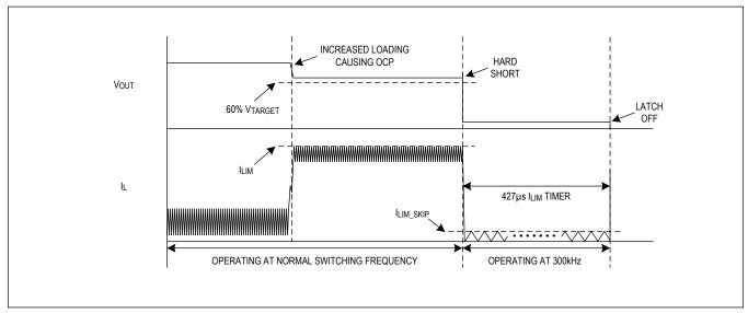
Figure 4. Overcurrent and Output Hard-Short Behavior
