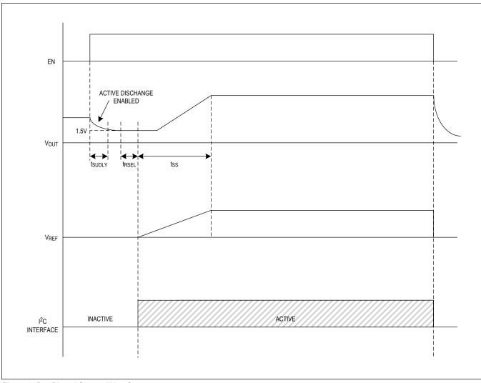
Figure 1. Pre-Biased Startup Waveform
