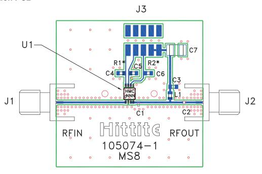
\* For 5V operation on Vctl line, select R1, R2 such that 3.6V is presented on Pins 6 and 8.
