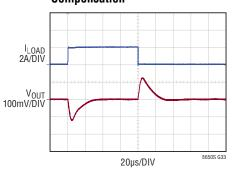
40mA TO 2A TRANSIENT  $3.3V_{OUT}$   $C_{OUT} = 47\mu F \times 2$ FCM,  $f_{SW} = 2MHz$
