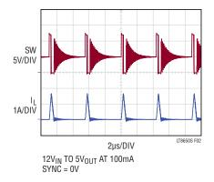
Figure 2. Burst Mode Operation
