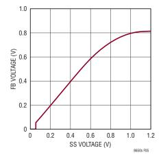
Figure 5. SS Pin Tracking
