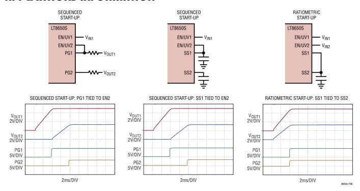
Figure 6. Sequencing and Start-Up Configurations
