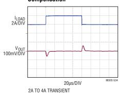
$3.3V_{OUT}$  $C_{OUT} = 47\mu F \times 2$ FCM,  $f_{SW} = 2MHz$   $C_C = 220pF$ ,  $R_C = 14k\Omega$
