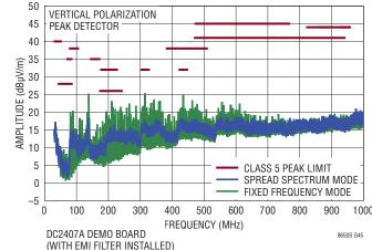
(WITH EMITFICIEN INSTACLED) 12V INPUT TO 5V OUTPUT1 AT 4A AND 3.3V OUTPUT2 AT 4A, f<sub>SW</sub> = 2MHz
