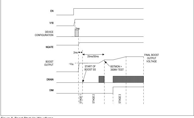
Figure 2. Boost Start-Up Waveforms
