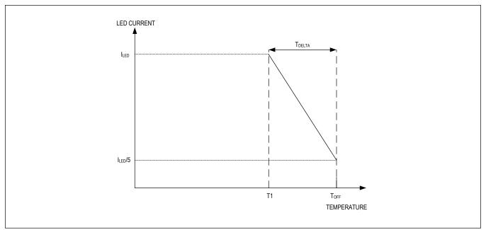
Figure 3. Temperature Foldback Curve
