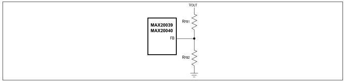
Figure 1. Setting the Output Voltage
