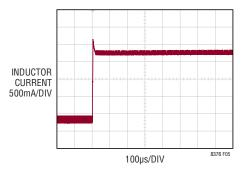
Figure 5. Extended Off-Time at Current Limit
