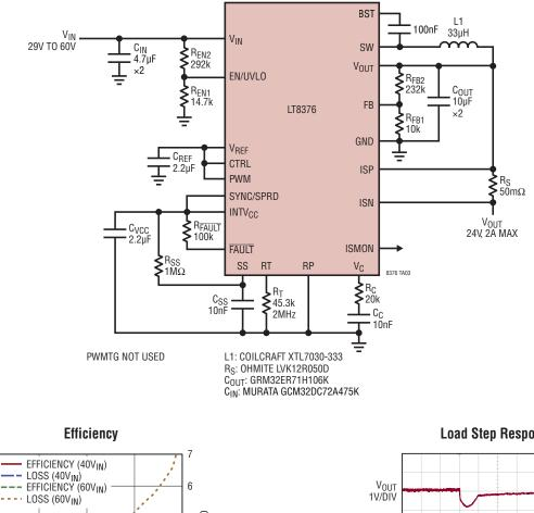
24V Voltage Regulator with Spread Spectrum
