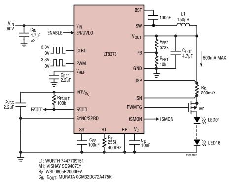
LED Driver with Duty Cycle LED Current
