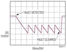
Figure 11. Hiccup Response to Fault
