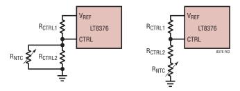
Figure 3. Setting CTRL with NTC Resistors
