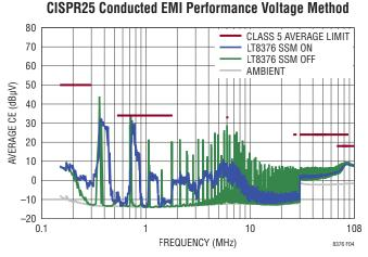
Figure 4. Typical Average Conducted Emissions
