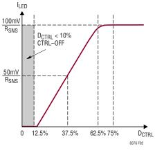
Figure 2. Duty Ratio CTRL Range
