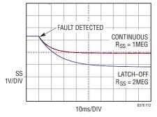
Figure 12. Latch-Off Response to a Fault
