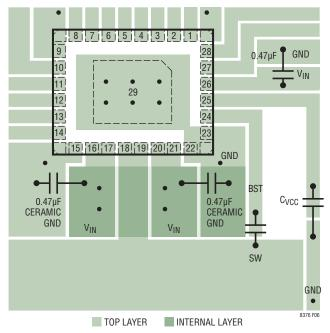
Figure 6. Placement of Input Capacitors
