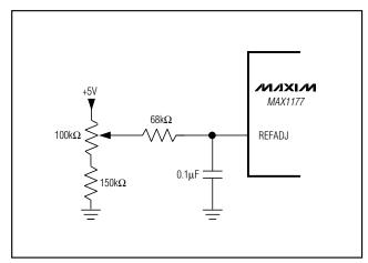
Figure 7. MAX1177 Reference Adjust Circuit
