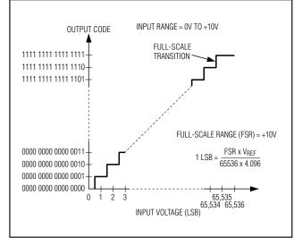
Figure 8. MAX1177 Transfer Function
