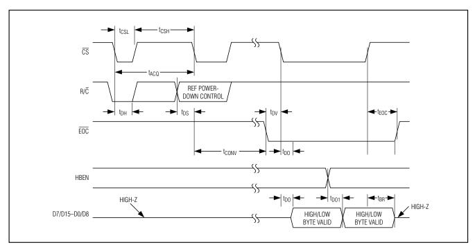
Figure 2. MAX1177 Timing Diagram
