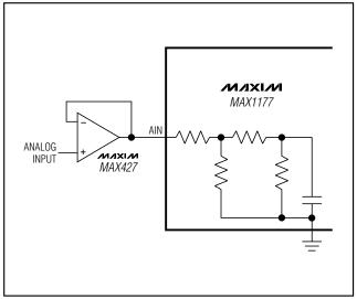
Figure 9. MAX1177 Fast-Settling Input Buffer
