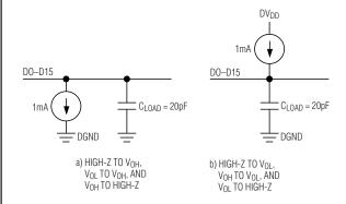
Figure 1. Load Circuits
