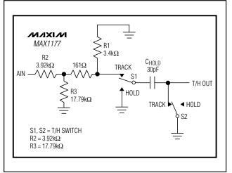
Figure 4. Equivalent Input Circuit
