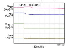
OPEN LED Protection: Keep Running Mode (R<sub>SS</sub> = 100k)
