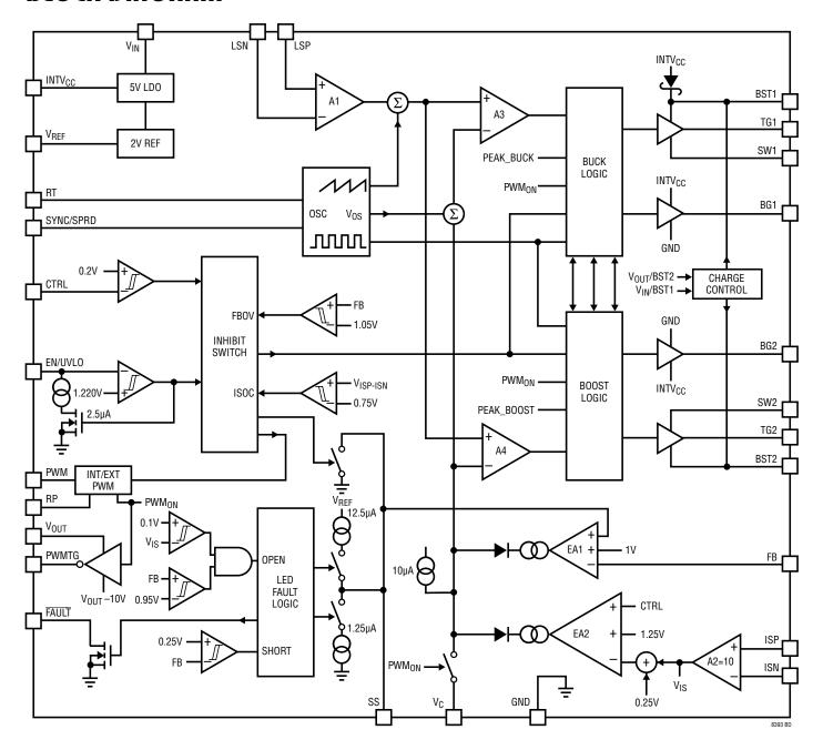
The LT8393 is a current mode LED controller that can regulate LED current from input voltages above, below, or equal to the LED string voltage. The ADI proprietary peak-buck peak-boost current mode control scheme uses a single inductor current sense resistor and provides smooth transition between the buck region, buck-boost region, and boost region. Its operation is best understood by referring to the Block Diagram.
