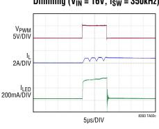
100Hz 500:1 External PWM Dimming ( $V_{IN} = 8V$ ,  $f_{SW} = 350kHz$ )
