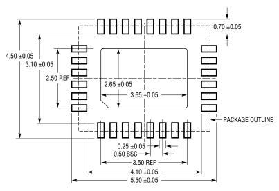
RECOMMENDED SOLDER PAD PITCH AND DIMENSIONS APPLY SOLDER MASK TO AREAS THAT ARE NOT SOLDERED
