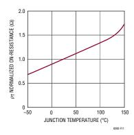
Figure 11. Normalized R<sub>DS(ON)</sub> vs Temperature
