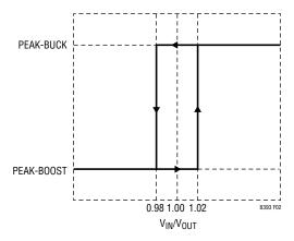
Figure 2. Current Mode vs V<sub>IN</sub>/V<sub>OUT</sub> Ratio
