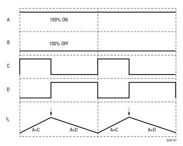
Figure 7. Peak-Boost in Boost Region (V<sub>IN</sub> << V<sub>OUT</sub>)
