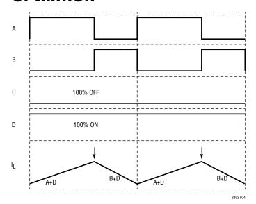
Figure 4. Peak-Buck in Buck Region (V<sub>IN</sub> >> V<sub>OUT</sub>)
