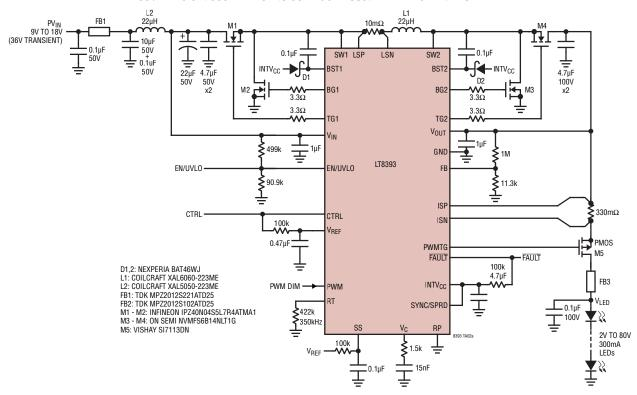
100Hz 1000:1 External PWM Dimming (V<sub>IN</sub> = 32V, f<sub>SW</sub> = 350kHz)
