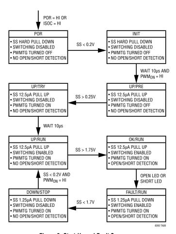
Figure 8. Start-Up and Fault Sequence
