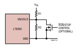
Figure 12. V<sub>IN</sub> Undervoltage Lockout (UVLO)
