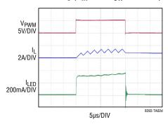
OPEN LED Protection: Hiccup Mode (R<sub>SS</sub> = Open)
