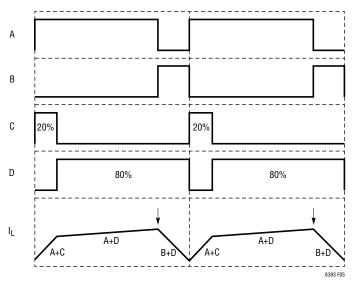
Figure 5. Peak-Buck in Buck-Boost Region (V<sub>IN</sub> ~> V<sub>OUT</sub>)
