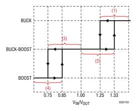
Figure 3. Operation Region vs V<sub>IN</sub>/V<sub>OUT</sub> Ratio
