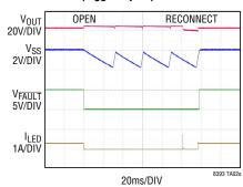
OPEN LED Protection: Latch-Off Mode (R<sub>SS</sub> = 499k)
