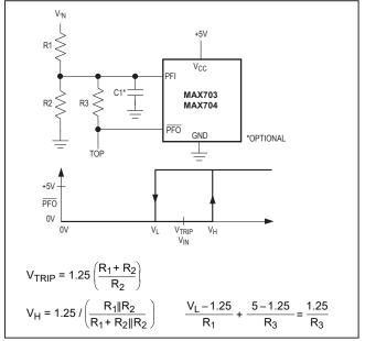
Figure 7. Adding Hysteresis to the Power-Fail Comparator
