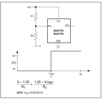
Figure 8. Monitoring a Negative Voltage
