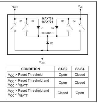
Figure 3. Battery-Switchover Block Diagram
