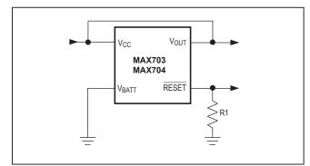
Figure 6. RESET Valid to Ground Circuit
