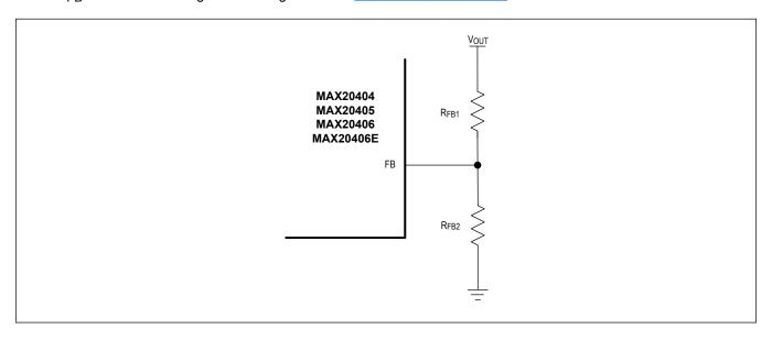
Figure 2. Output Voltage Setting Using External Resistor-Divider
