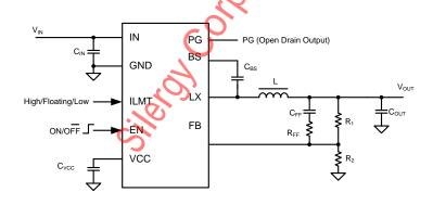
Figure 1 Schematic
