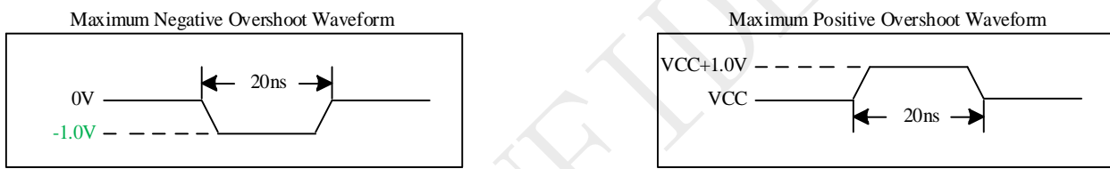
Figure 5-1 Maximum Overshoot Waveform
