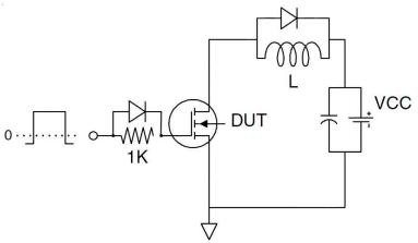
3) Switch Time Test Circuit
