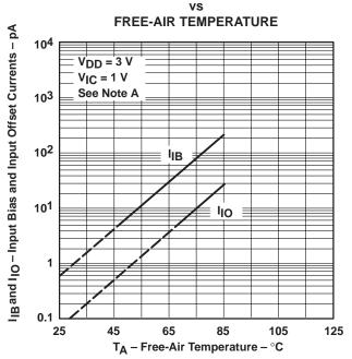
NOTE: The typical values of input bias current and input offset current below 5 pA were determined mathematically.
