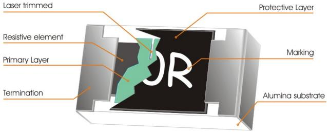
Fig 1. Construction of Chip-R
