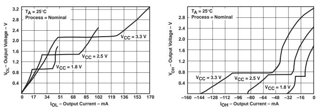
Figure 1. Output Voltage vs Output Current
