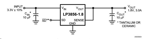
\*\* $\overline{\text{SD}}$  pin must be pulled high through a 10k $\Omega$  pull-up resistor. See Application Hints for more information.
