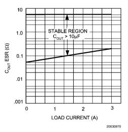
FIGURE 1. ESR Curve for  $C_{OUT}$  (with 10µF Tantalum Input Capacitor)
