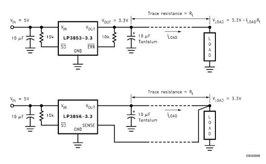
FIGURE 4. Improving remote load regulation using LP3856
