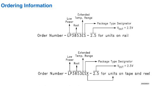
Package Type Designator is "T" for TO220 package, and "S" for TO263 package.
