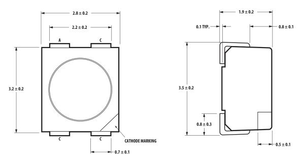
NOTE: All dimensions in millimeters. Electrical connection between all cathodes is recommended.
