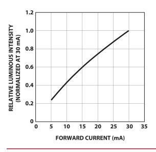
Figure 4: Relative Intensity vs. Forward Current (AllnGaP)
