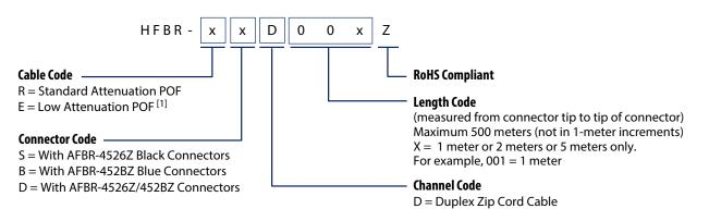
1. Standard (type = "R") and Low Attenuation (type = "E") cables comply with UL VW-1 flame retardant specification (UL file # E89328). Note: For other cable lengths please contact a Broadcom representative.
