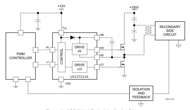
Figure 18. UCC27211A Typical Application Diagram
