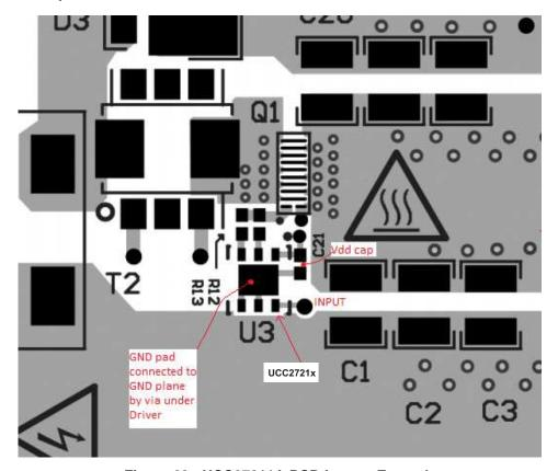
Figure 23. UCC27211A PCB Layout Example
