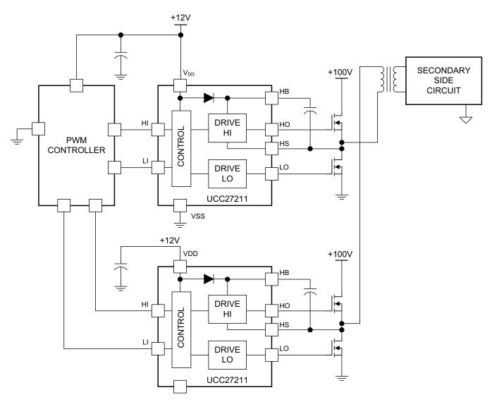
Figure 19. UCC27211 Typical Application Diagram
