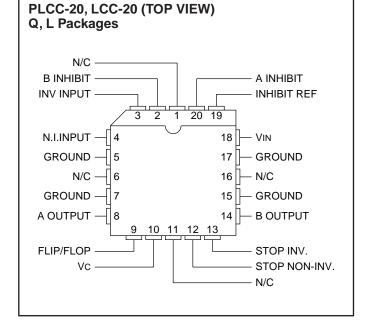
Note: All four ground pins must be connected to a common ground.
