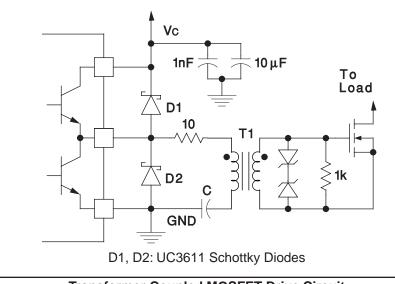
**Transformer Coupled MOSFET Drive Circuit**
