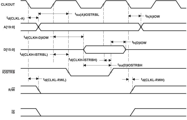
Figure 19. Parallel I/O Port Write (IOSTRB = 0)
