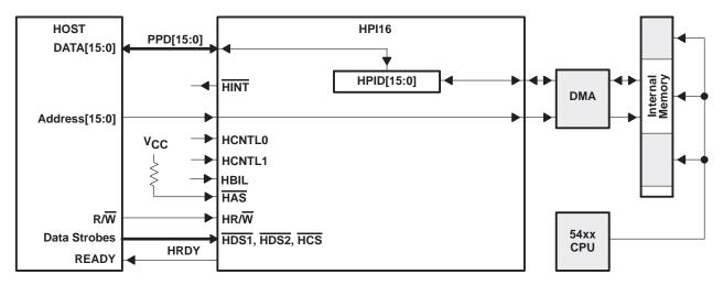
Figure 7. Host-Port Interface — Nonmultiplexed Mode
