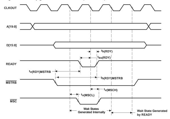
Figure 21. Memory Write With Externally Generated Wait States
