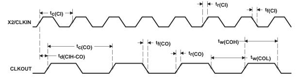
Figure 14. External Divide-by-Two Clock Timing
