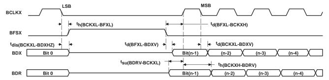
Figure 35. McBSP Timing as SPI Master or Slave: CLKSTP = 11b, CLKXP = 0
