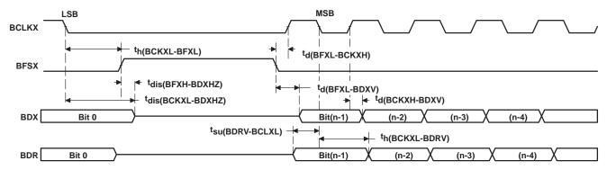
Figure 34. McBSP Timing as SPI Master or Slave: CLKSTP = 10b, CLKXP = 0
