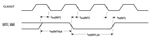
Figure 26. Interrupt Timing
