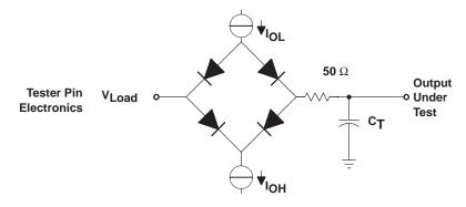
Where:  $I_{OL}$  = 1.5 mA (all outputs)  $I_{OH}$  = 300  $\mu$ A (all outputs)
