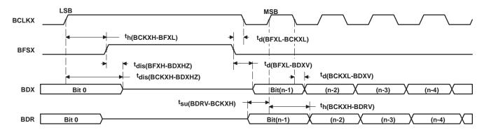
Figure 36. McBSP Timing as SPI Master or Slave: CLKSTP = 10b, CLKXP = 1
