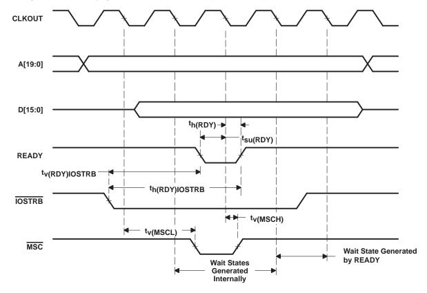
Figure 23. I/O Write With Externally Generated Wait States
