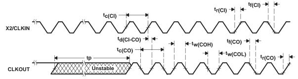
Figure 15. External Multiply-by-One Clock Timing
