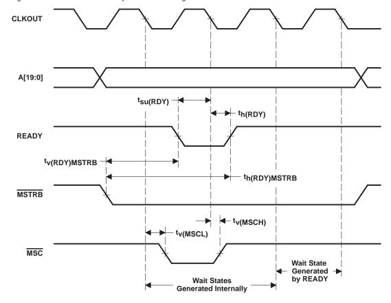
Figure 20. Memory Read With Externally Generated Wait States
