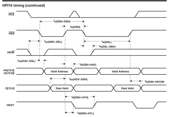
Figure 43. Nonmultiplexed Write Timings
