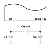
Figure 13. Internal Oscillator With External Crystal
