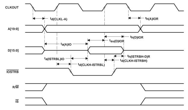
Figure 18. Parallel I/O Port Read (IOSTRB = 0)
