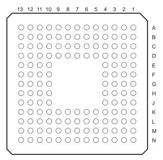
The pin assignments table to follow lists each signal quadrant and BGA ball number for the TMS320UC5409GGU (144-pin BGA package).
