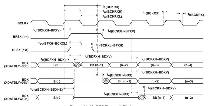
Figure 32. McBSP Transmit Timings
