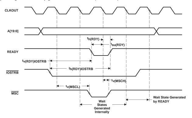
Figure 22. I/O Read With Externally Generated Wait States
