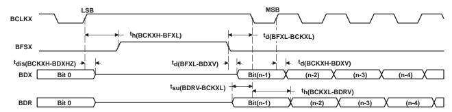
Figure 37. McBSP Timing as SPI Master or Slave: CLKSTP = 11b, CLKXP = 1
