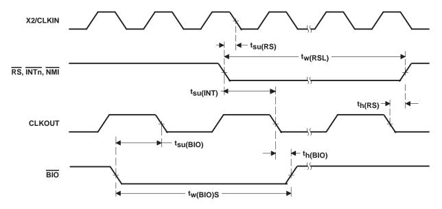
Figure 25. Reset and BIO Timings
