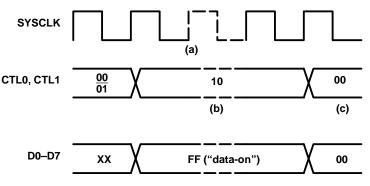
Figure 19. Null Packet Reception Timing
