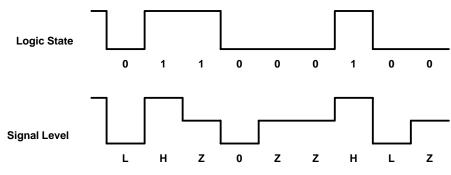
Figure 14. Signal Transformation for Digital Differentiation
