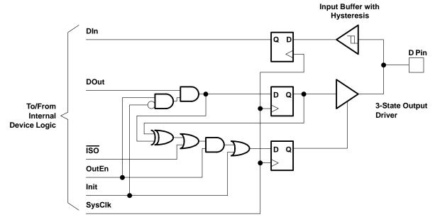
Figure 15. Input/Output Differentiation Logic
