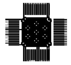
Figure 10. Example of a Thermal Land for the TSB41LV02A PHY
