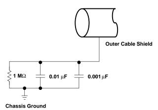
Figure 5. Typical Compliant DC Isolated Outer Shield Termination
