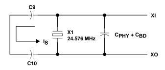
Figure 11. Load Capacitance for the TSB41LV02A PHY
