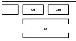
Figure 12. Recommended Crystal and Capacitor Layout
