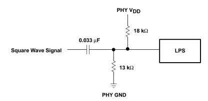
Figure 8. Isolated Circuit Connection for LPS
