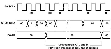
Figure 21. Cancelled/Null Packet Transmission
