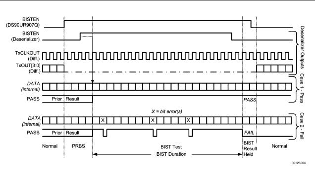
FIGURE 26. BIST Waveforms
