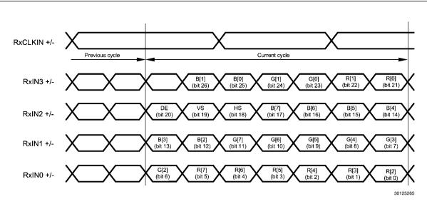
FIGURE 20. 8-bit Channel Link Mapping: LSB's on RxIN3
