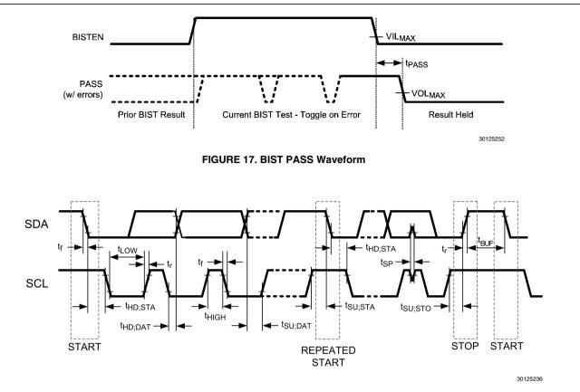
FIGURE 18. Serial Control Bus Timing Diagram
