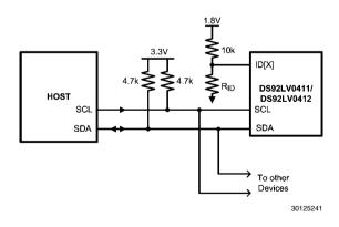
FIGURE 27. Serial Control Bus Connection
