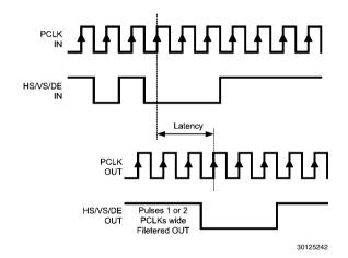
FIGURE 22. Video Control Signal Filter Wavefrom
