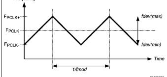
FIGURE 24. SSCG Waveform
