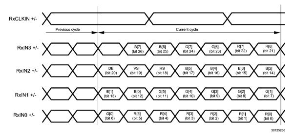
FIGURE 21. 8-bit Channel Link Mapping: MSB's on RxIN3
