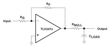
Figure 42. Driving a Capacitive Load
