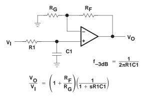
Figure 44. Single-Pole Low-Pass Filter
