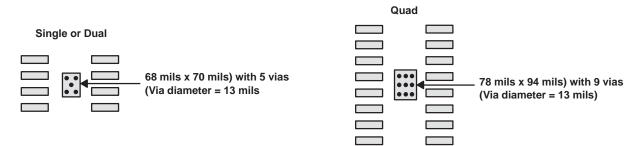
Figure 47. PowerPAD PCB Etch and Via Pattern
