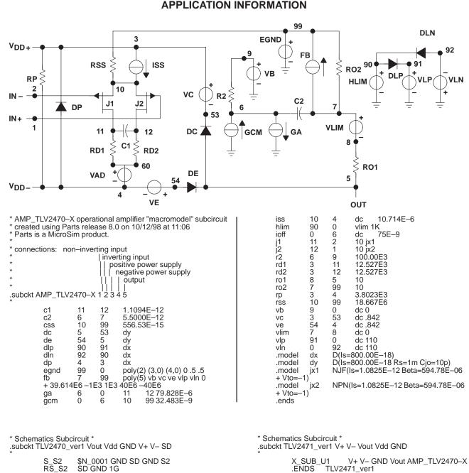
.MODEL S2 VSWITCH Roff=1e6 Ron=1.0 Voff=0.0 + Von=1.0 S\_S1 \$ \$N\_0002 VDD SD GND S1 RS S1 SD GND 1G .MODEL S1 VSWITCH Roff=1e6 Ron=1.0 Voff=0.0 + Von=1.0 S\_S3 V Vout \$N\_0003 SD GND S3 RS\_S3 SD GND 1G .MODEL S3 VSWITCH Roff=1e6 Ron=1.0 Voff=0.0 + Von=1.0 X\_SUB\_U1 V+ V- \$N\_0002 \$N\_003 + AMP\_TLV2470-X .ENDS TLV2470\_ TLV2470\_ver1
