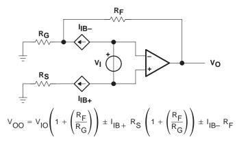
Figure 43. Output Offset Voltage Model
