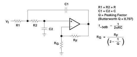
Figure 45. 2-Pole Low-Pass Sallen-Key Filter
