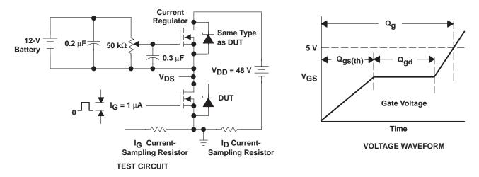
Figure 3. Gate-Charge Test Circuit and Voltage Waveform
