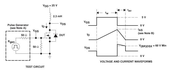
NOTES: A. The pulse generator has the following characteristics:  $t_r \le 10$  ns,  $t_f \le 10$  ns,  $t_{O} = 50 \Omega$ .
