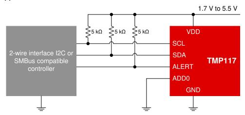
Figure 8-1. Typical Connections
