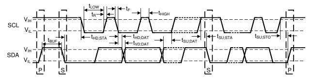
Figure 6-1. Two-Wire Timing Diagram
