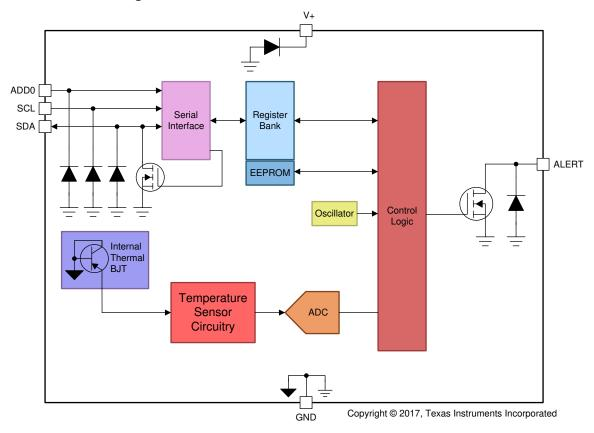
Figure 7-1. Internal Block Diagram
