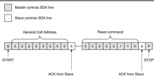
Figure 7-12. General-Call Reset Command Timing Diagram
