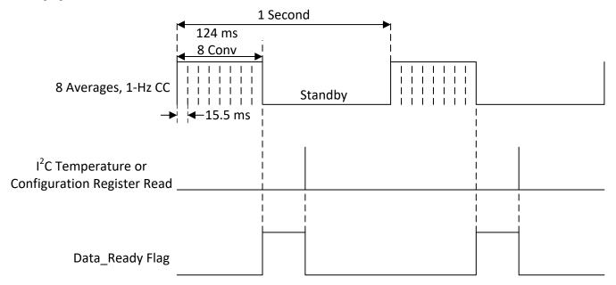
Figure 7-2. Averaging Timing Diagram
