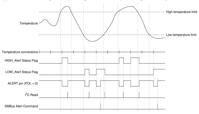
Figure 7-5. Alert Mode Timing Diagram
