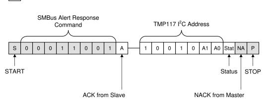
Figure 7-11. SMBus ALERT Timing Diagram
