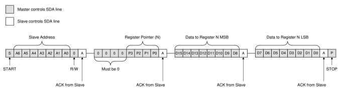
Figure 7-9. Write Word Command Timing Diagram
