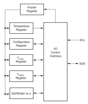
Figure 7-8. Internal Register Structures
