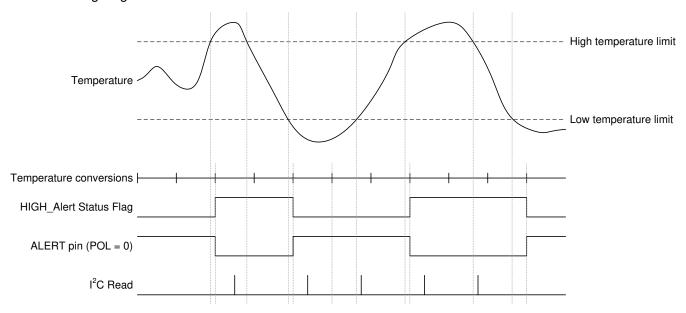
Figure 7-6. Therm Mode Timing Diagram
