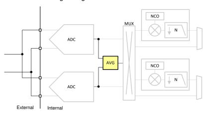
Figure 8-50. Digital Channel Averaging Diagram
