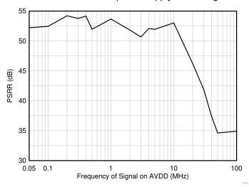
Figure 9-7. Power supply rejection ratio (PSRR) vs frequency
