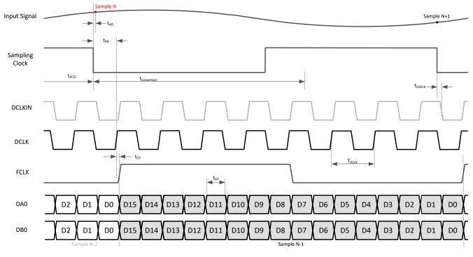
Figure 7-2. Timing diagram: 1-wire SLVDS (default output bit mapper)
