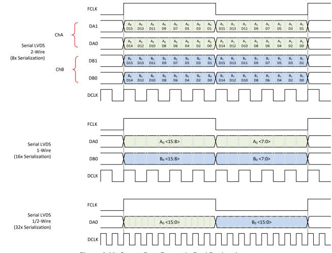
Figure 8-39. Output Data Format in Real Decimation
