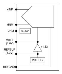
Figure 8-17. Different voltage reference options for ADC366x
