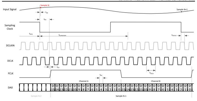
Figure 7-3. Timing diagram:1/2-wire SLVDS (default output bit mapper)
