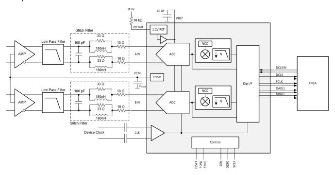
Figure 9-1. Typical configuration for a spectrum analyzer with DC support
