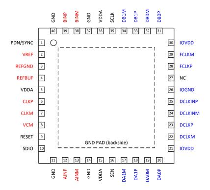
Figure 5-1. RSB (WQFN) Package, 40-Pin (Top View)
