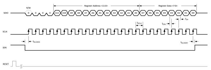
Figure 8-52. Serial Register Write Timing Diagram
