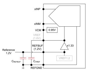
Figure 8-20. External 1.2V reference using internal reference buffer
