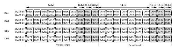
Figure 8-42. 2-wire output bit mapper
