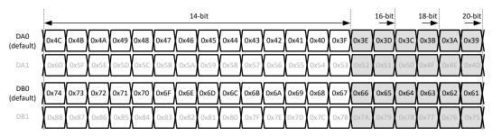
Figure 8-44. 1-wire output bit mapping
