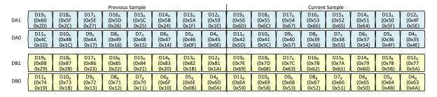
Figure 8-43. Example: 2-wire output bit mapping
