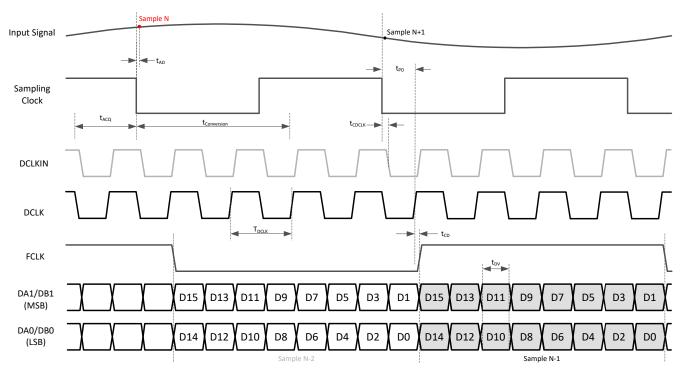
Figure 7-1. Timing diagram: 2-wire SLVDS (default output bit mapper)
