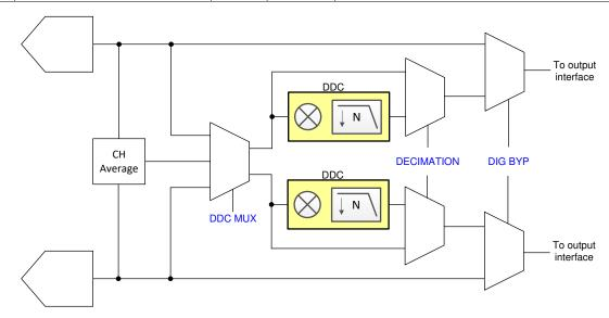
Figure 8-69. Register control for digital features
