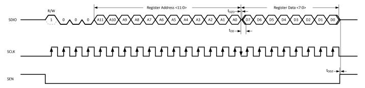
Figure 8-53. Serial Register Read Timing Diagram
