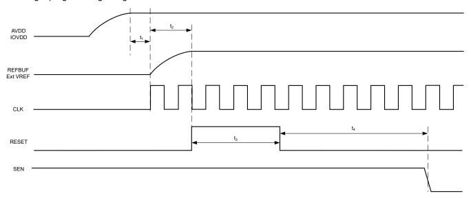
Figure 9-6. Initialization of serial registers after power up
