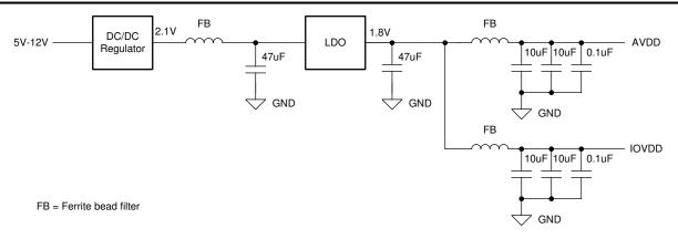
Figure 9-8. Example: LDO Linear Regulator Approach
