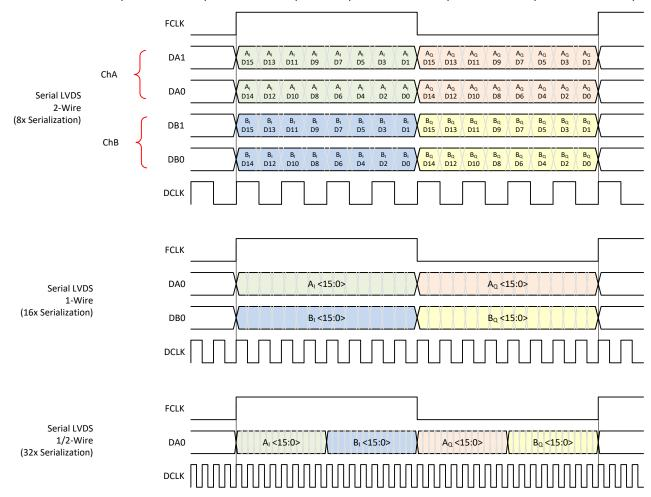
Figure 8-38. Output Data Format in Complex Decimation
