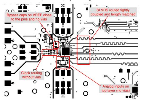
Figure 9-10. Layout example: top layer of ADC366x/368x EVM
