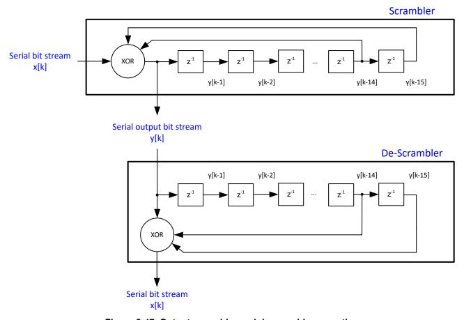
Figure 8-47. Output scrambler and descrambler operation
