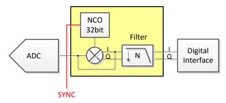
Figure 8-21. Internal Digital Decimation Filter
