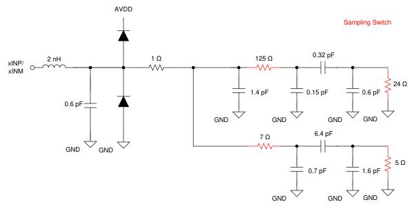
Figure 8-1. Equivalent Input Network
