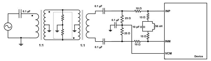
Figure 204. Driving Circuit for Mid-Range Input Frequencies (100 MHz < fin < 230 MHz)
