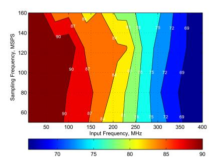
Figure 139. Spurious-Free Dynamic Range (SFDR) for 0-dB Gain
