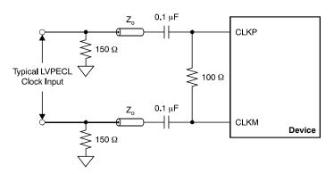
Figure 150. LVPECL Clock Driving Circuit
