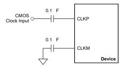
Figure 152. Single-Ended Clock Driving Circuit
