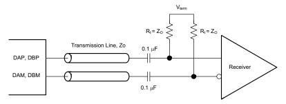
Figure 159. CML Output Connections
