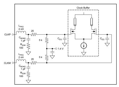
NOTE: C<sub>EQ</sub> is 1 pF to 3 pF and is the equivalent input capacitance of the clock buffer.
