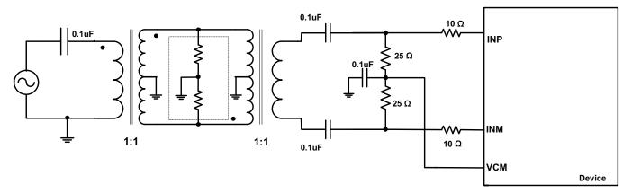
Figure 206. Driving Circuit for High Input Frequencies (f<sub>IN</sub> > 230 MHz)
