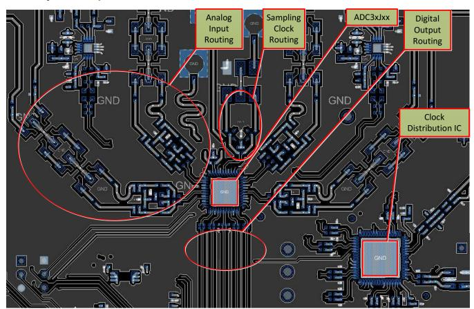
Figure 208. Typical Layout of the ADC34J2x Board
