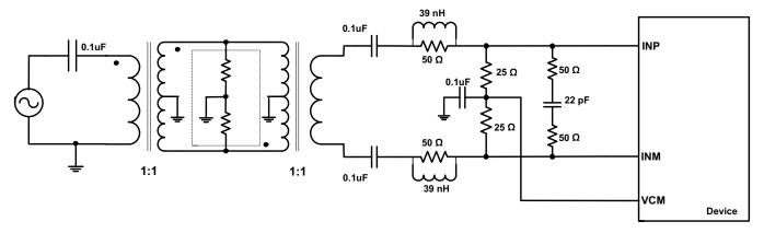
Figure 202. Driving Circuit for Low Input Frequencies
