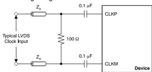
Figure 149. LVDS Clock Driving Circuit
