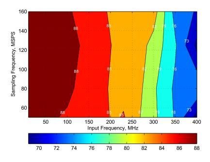
Figure 140. Spurious-Free Dynamic Range (SFDR) for 6-dB Gain
