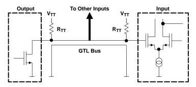
Figure 3. GTL Bus: An Open-Drain Bus
