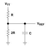
Figure 4. Suggested Connection of V<sub>REF</sub> Terminal
