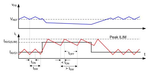
Figure 8-1. Current Limit Timing Diagram
