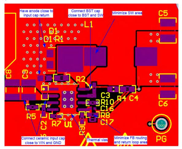
Figure 9-14. LM5013 Layout Example
