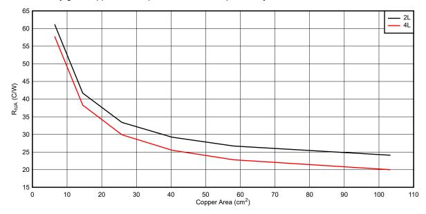
Figure 9-15. Typical R<sub>OJA</sub> vs Copper Area
