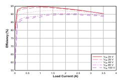
Typical Application Efficiency, V<sub>OUT</sub> = 12 V
