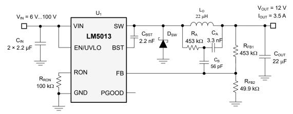
Figure 9-1. Typical Application,  $V_{IN(nom)}$  = 48 V,  $V_{OUT}$  = 12 V,  $I_{OUT(max)}$  = 3.5 A,  $f_{SW(nom)}$  = 300 kHz
