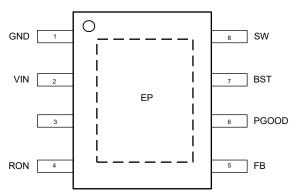
Figure 6-1. 8-Pin SO PowerPAD<sup>™</sup> DDA Integrated Circuit Package (Top View)
