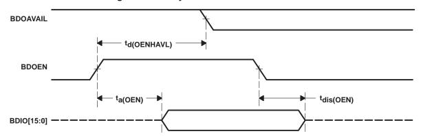
Figure 9-11. Asynchronous Burst Mode Read
