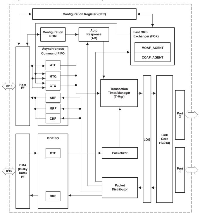
Figure 2-1. Functional Block Architecture
