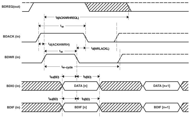
NOTE: t<sub>d</sub>(ACKHREQL) is the duration from when both BDACK and BDWR / BDRD are asserted (rising edge) until BDREQ is negated (falling edge). BDREQ remains active (asserted) while the FIFO has capacity.
