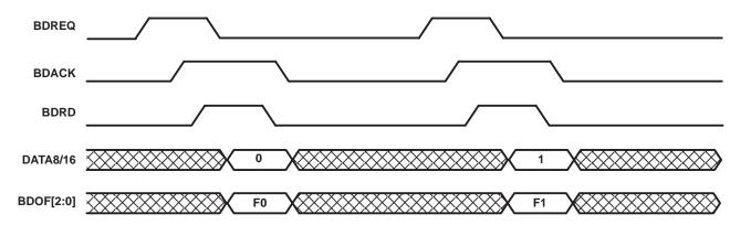
In this mode, data is output on the BDRD falling edge.
