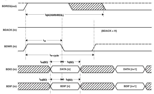
NOTE: t<sub>d(ACKHREQL)</sub> is the duration from when both BDACK and BDWR / BDRD are asserted (rising edge) until BDREQ is negated (falling edge). BDREQ remains active (asserted) while the FIFO has capacity.
