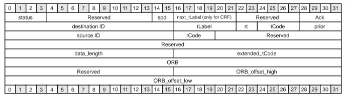
Figure 4–13. MRF/CRF Receive Long Format (ORB)
