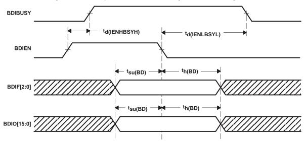
Figure 9-8. Asynchronous Handshake Mode Write
