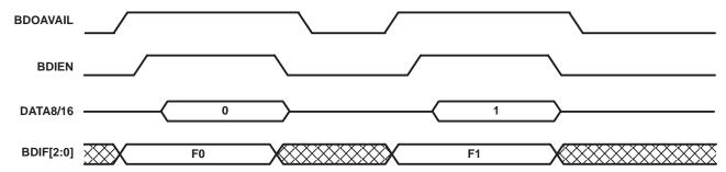
The data is output by repeating BDOEN low and high. BDOEN is asserted after confirming the BDOAVAIL input is true.
