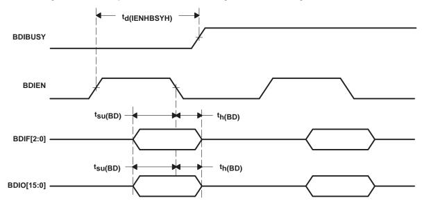
Figure 9-10. Asynchronous Burst Mode Write
