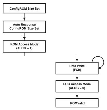
Figure 5-2. ConfigROM Setup
