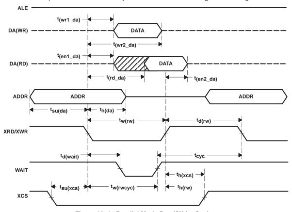
Figure 10-1. Parallel Mode Read/Write Cycle
