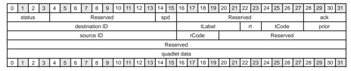
Figure 4–9. Generic Receive Format of Packet With Quadlet Data
