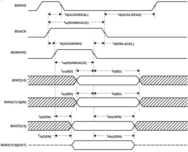
NOTE:  $t_{d(ACKHREQL)}$  is the duration from when both BDACK and BDWR / BDRD are asserted (rising edge) until BDREQ is negated (falling edge).  $t_{d(ACKLREQH)}$  is the duration from when both BDACK and BDWR / BDRD are negated (falling edge) until BDREQ is asserted (rising edge).
