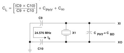
Figure 12-4. Load Capacitance for the TSB43AA82 PHY Portion
