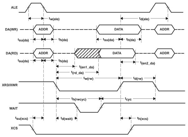
Figure 10-2. Multiplex (MUX) Mode Read/Write Cycle
