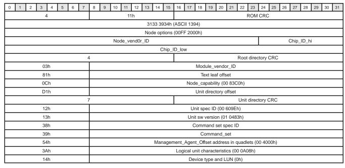
Figure 5-1. Example ConfigROM Base Structure (Reference SBP-2 Draft)
