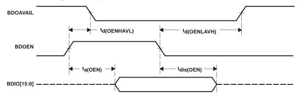
Figure 9-9. Asynchronous Handshake Mode Read
