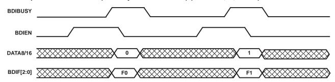
The data needs to be specified by the BDIEN falling edge. Also, BDIEN needs to be asserted after confirming BDIBUSY input is false.
