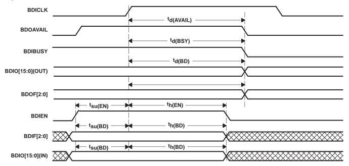
Figure 9-1. Synchronous Mode
