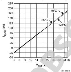
Input Bias Current Over Temperature (A2 Inputs)
