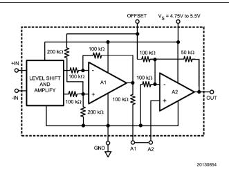
FIGURE 3. Mid-Rail Offset Adjustment Pin Schematic
