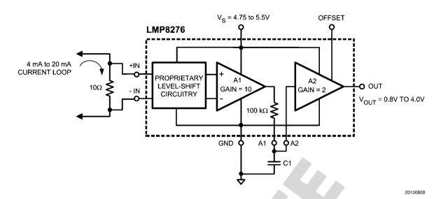
FIGURE 8. Current Loop Receiver
