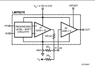
FIGURE 6. Gains Less Than 20
