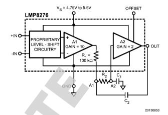
FIGURE 5. Low-Pass Filter With LMP8276
