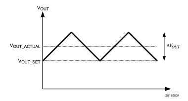
It can be seen that the average output voltage  $(V_{OUT\_ACTUAL})$  is higher than the output voltage  $(V_{OUT\_SET})$  that was calculated by the earlier equation by exactly half the output voltage ripple. The output voltage that is targeted for regulation may then be appended according to the voltage ripple. This can be seen below:
