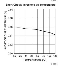
**Typical Performance Characteristics** All curves taken at VIN = 3.3V with configuration in typical application circuit shown in Application Information section of this datasheet. T<sub>J</sub> = 25°C, unless otherwise specified. (Continued)
