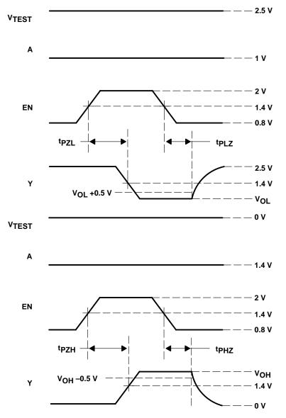
Figure 3. Enable/Disable Time Test Circuit and Wave Forms
