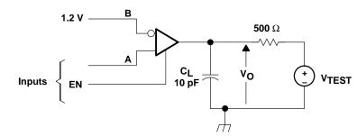
NOTE A: All input pulses are supplied by a generator having the following characteristics:  $t_r$  or  $t_f \le 1$  ns, pulse repetition rate (PRR) = 0.5 Mpps, pulse width = 500 ± 10 ns. C<sub>L</sub> includes instrumentation and fixture capacitance within 0,06 m of the D.U.T.
