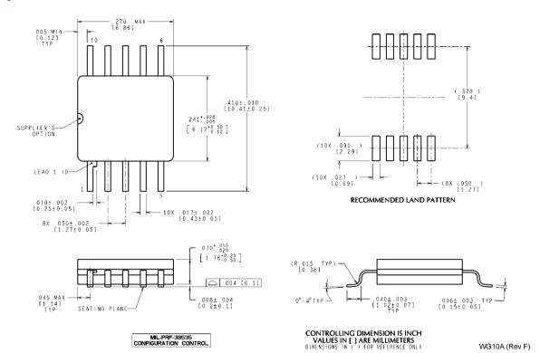
10-Pin Ceramic SOIC NS Package Number WG10A
