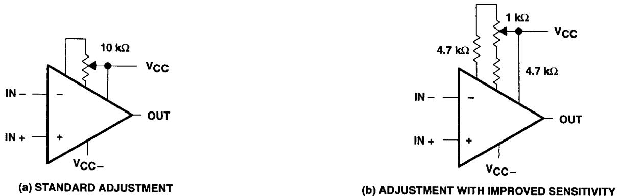
Figure 47. Input Offset-Voltage Nulling Circuits
