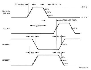
FIGURE 4. Propagation Delay (Reset)
