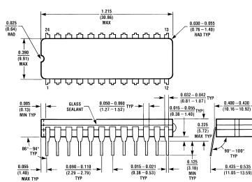
24-Lead Ceramic Dual-In-Line Package (0.400" Wide) (D) NS Package Number J24E
