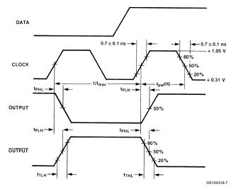
FIGURE 3. Propagation Delay (Clock) and Transition Times
