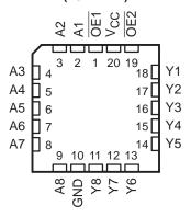
The 3-state control gate is a two-input AND gate with active-low inputs so that if either output-enable ( $\overline{OE1}$  or  $\overline{OE2}$ ) input is high, all corresponding outputs are in the high-impedance state. The outputs provide inverted data when they are not in the high-impedance state.
