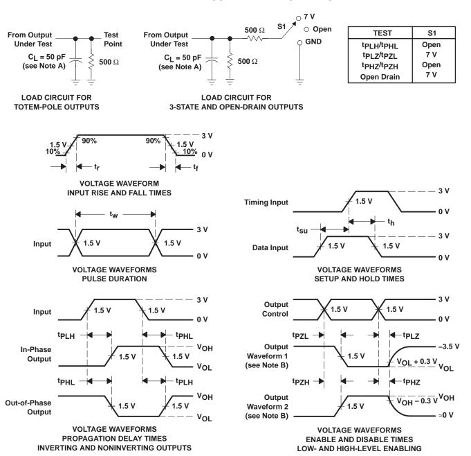
NOTES: A. C<sub>I</sub> includes probe and jig capacitance.
