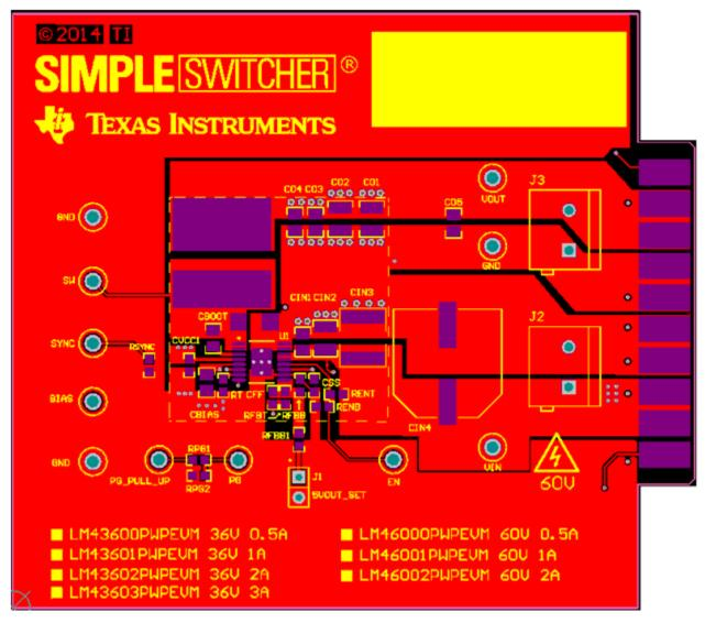
Figure 3. Top Assembly Layer
