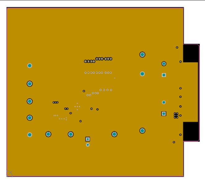
Figure 5. Mid Layer 1 Ground Plane
