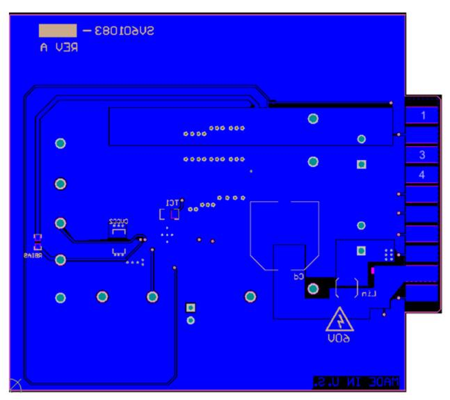
Figure 7. Bottom Layer Routing
