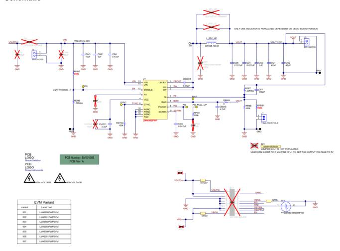
Figure 2. LM46002EVM Schematic
