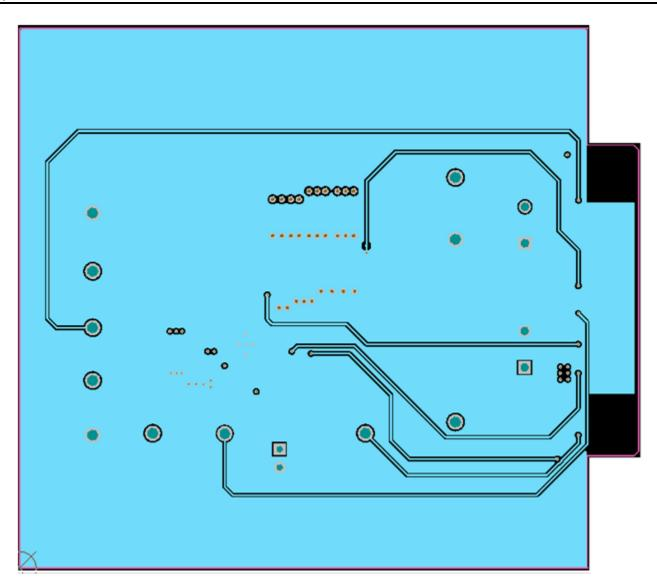
Figure 6. Mid Layer 2 Routing
