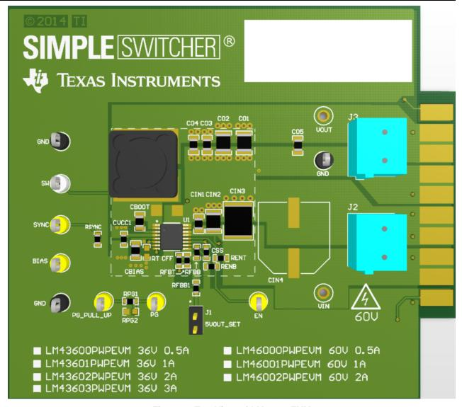
Figure 1. Top View of LM46002EVM
