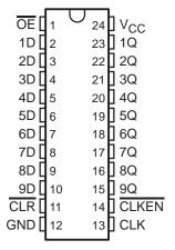
The nine flip-flops are edge-triggered D-type flip-flops. With the clock-enable (CLKEN) input low, the flip-flops store data on the low-to-high transitions of the clock. Taking CLKEN high disables the clock buffer, thus latching the outputs. The SN74BCT29823 has noninverting data (D) inputs. Taking the clear (CLR) input low causes the nine Q outputs to go low independent of the clock.
