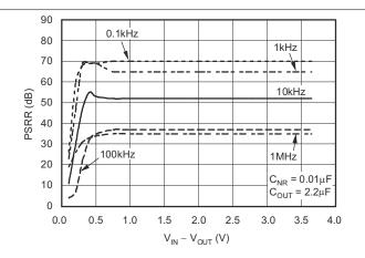
Figure 6-7. Power-Supply Ripple Rejection vs  $V_{\text{IN}}$  –  $V_{\text{OUT}}$ ,  $I_{\text{OUT}}$  = 1 mA
