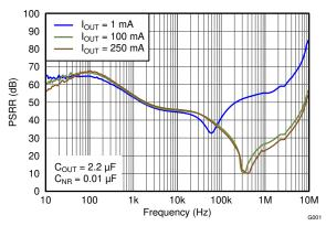
Figure 8-3. Power-Supply Rejection Ratio vs Frequency
