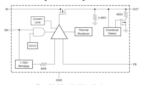
Figure 7-2. Adjustable-Voltage Version
