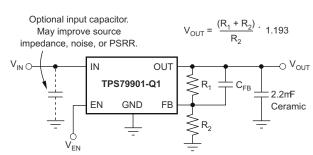
Typical Application Circuit Adjustable Voltage Version
