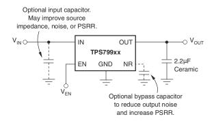
Figure 8-1. Typical Application Circuit for Fixed-Voltage Version
