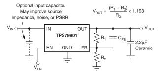
Figure 8-2. Typical Application Circuit for Adjustable-Voltage Version
