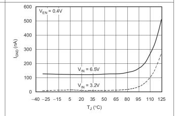
Figure 6-5. Ground Pin Current vs Input Voltage
